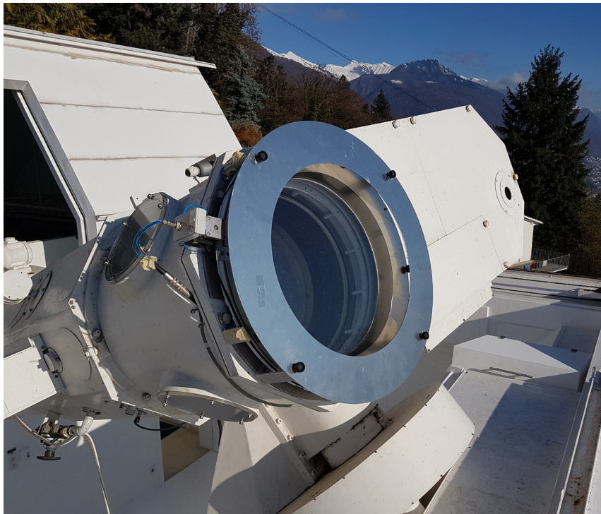
Figure 1. The Telescope Calibration Unit mounted in front of the IRSOL telescope.
